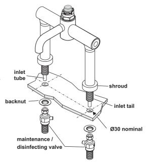
Figure 2 Installation - panel mounting
