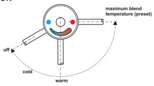
Figure 5 Showing the handle control positions.
